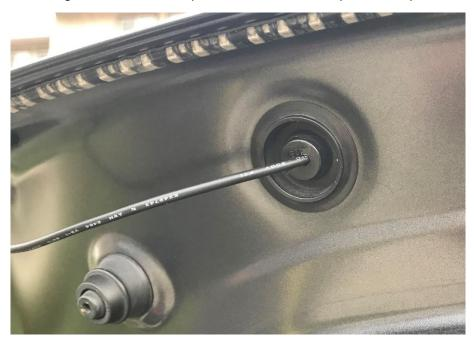
Insert the cable through the slit on the caps and install all the caps back in place.
