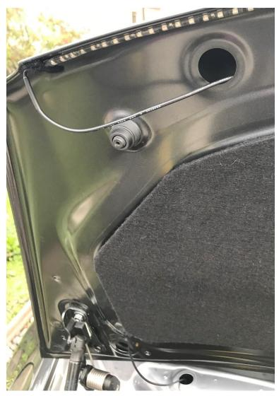
Connect the 2 pin connector from the cable to the harness.
