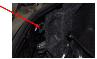
Remove one fastener and partially peel back the trunk side trim
